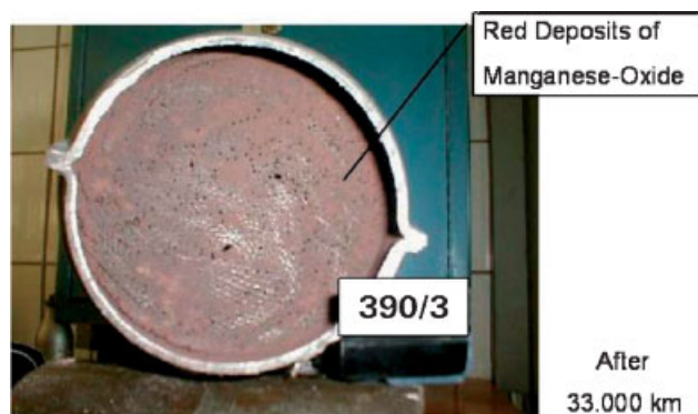
FIGURE 8. Experience with MMT. China: Blocked catalytic converter. Source: Schindler [2004].
