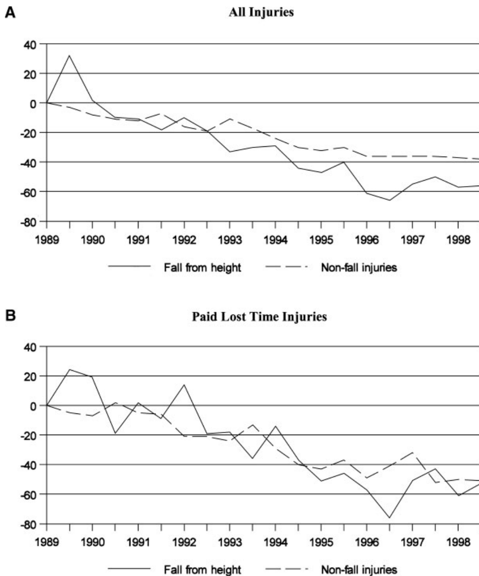
FIGURE 1. Percentages of change in injury rates over time, 1989–1998, Union Carpenters Washington State. A: All injuries. B: Paid lost time injuries.
